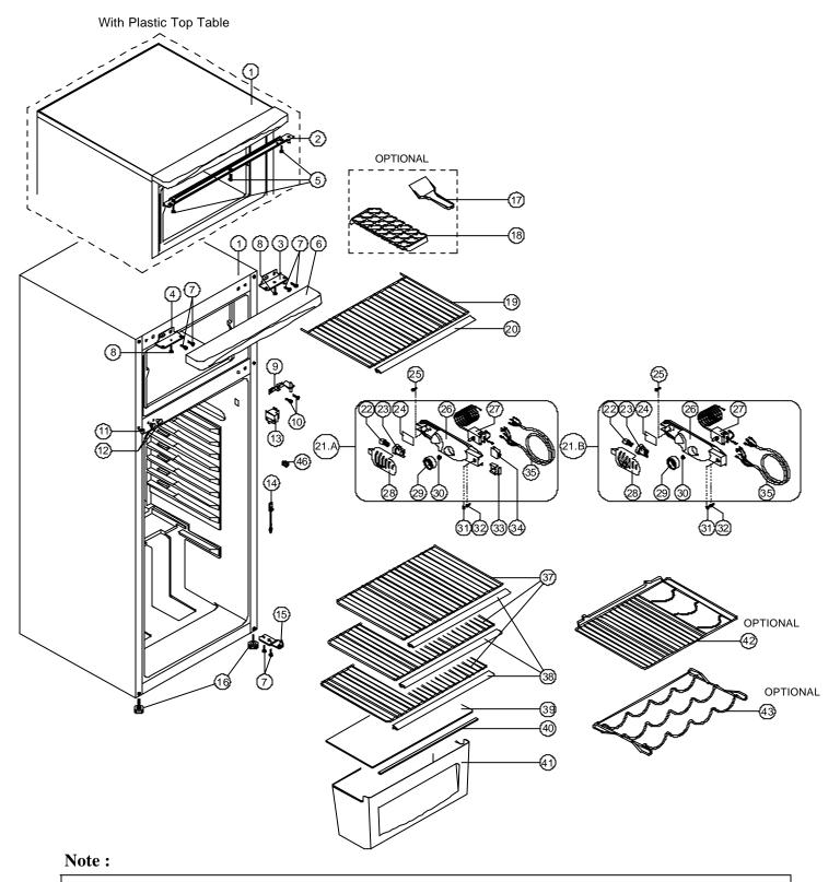
\*\*\* Thermostat Box Assy/260 (21.A) is used for products that are produced before 06.11.2002
