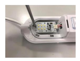
Disconnect the connector and change the led.
