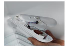
Firstly take off the button and screw and then take off all cable connection and pull thermostat bulb out
