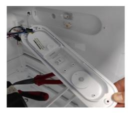
Place the thermostat, screws is tightened, insert the button Connect cables as shown below
