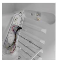
Take off the lamp cover, cable connection and screw at below picture
