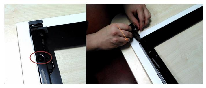
Disassemble removable inner glass spring as below,
