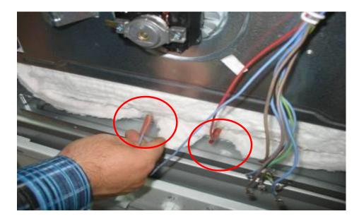
Raise the isolation wool softly upwards, remove the left and right screws which are connects bottom heater protection sheet metal to oven.
