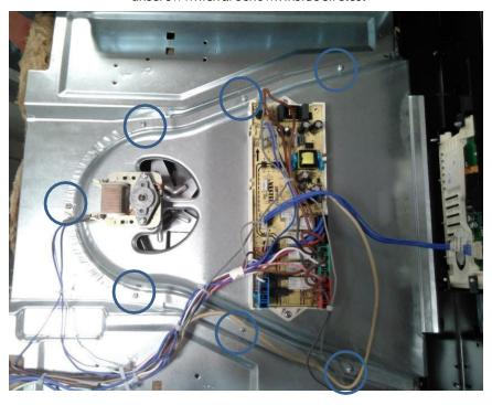
$Detach \, the \, nut \, by \, turning \, counterclockwise$
