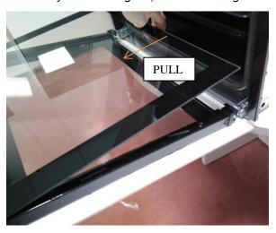
Unscrew as below to disassemble door profile.
