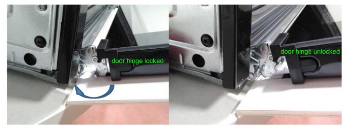
After unlock the hinge, pull and free the door as below.
