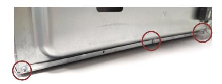
Disassemble the terminal box by pushing clips with screwdriver as below and assemble to new rear panel.
