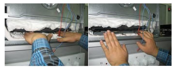
Pull out the bottom heater by raising it to upwards softly.
