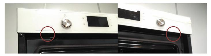
Remove the knobs by pulling.
