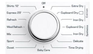
\*\*\*The machine has humidity sensor that detects whether the laundry dry or not. At the programs that work with humidity sensor laundry does not dry in fixed time. Duration is constantly updates according to humidity data taking from laundry.
