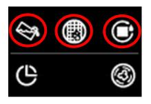
The case in the photo don't show us a failure code. (If it is don't blinking) Normally, when the drying program ends, the filter, water tank and end led are flashing. In addition, condenser cleaning warning led is on every 30 cycles.
