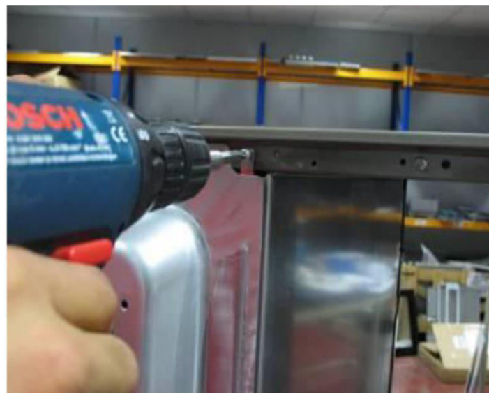
5-Unscrew the rear panel
