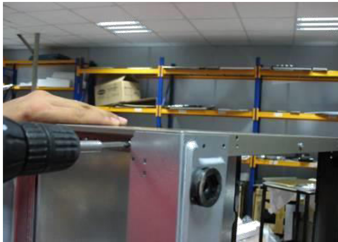
5-Unscrew the rear panel
