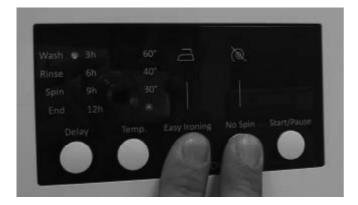
2. L4 and L5 will make fast blink for 2 sec to indicate child lock is activated.
