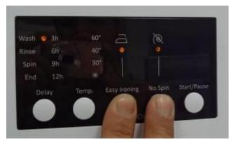
2. L4 and L5 will make fast blink for 2 sec to indicate child lock is activated.
