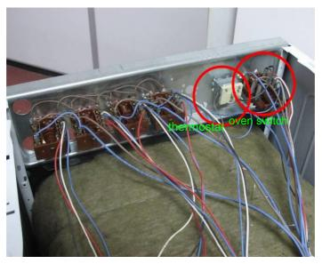
Remove wiring connections by a nipper
