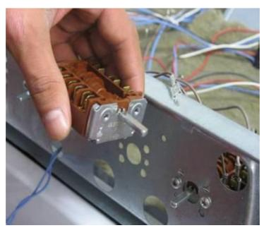
Do not compress the bottom plates of switch! **6-**In this case, you may cause short circuit and switch may not work correctly.
