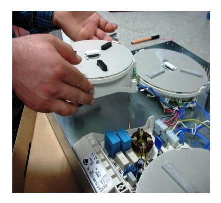
To change the touch control unit; remove connected wirings
