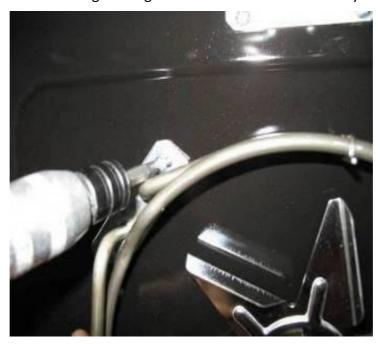
Pull out the wiring connections manually. The ring heater will be free then.
