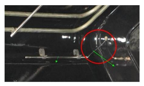
Manually remove thermostat bulb out of its brackets.
