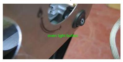
Attention: Do not push back the front panel hardly and fast; this may cause the button wirings get harmed. Please hold it until you take off the terminal contacts.
