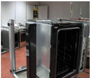
Repeat the same procedure backwards when assemblying the new side panel
