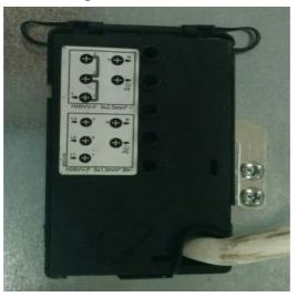
Press on the hooks of connection unit for opening terminal box.
