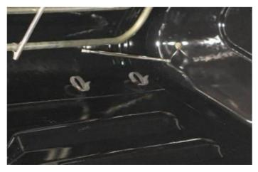
Now it is safe to pull back and remove thermostat bulb from the rear outlet.
