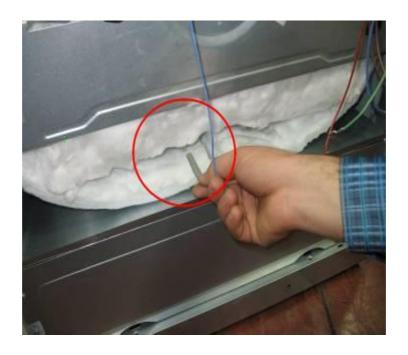
**2-**Take up the wrapping insulation (rockwool) slightly, then unscrew the right and left connections of bottom heating element.
