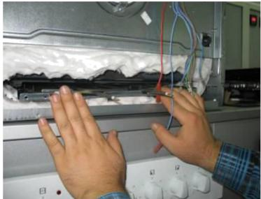
**4-**Hold up the heating element slightly and take out.
