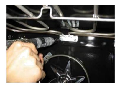
Pull out the wiring connections manually. The ring heater will be free then.
