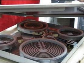
Remove the terminals of heating element that you want to change. (by a nipper)
