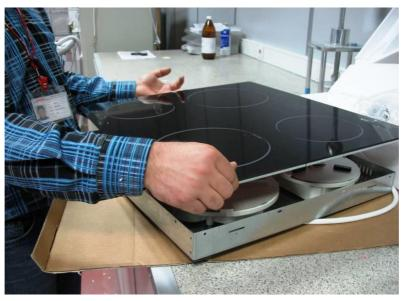
Pull off terminal connections on the heating element ( IHE )
