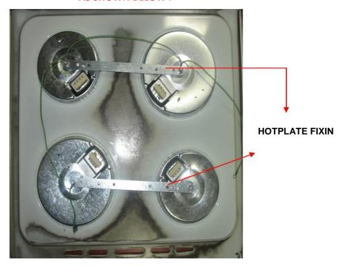
Ø 8 hotplate housing earthing vent is <u>moved</u> on the new cookers. We do no recommend to use hotplate fixing brackets on old cookers.
