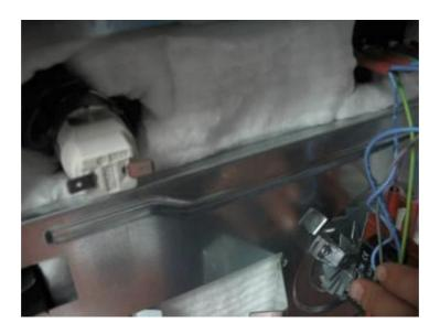
**3**-Press the hooks on the oven light (by a screwdriver) and then push into the cavity.
