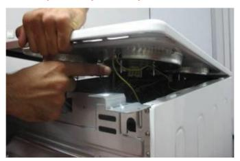
**3-**Take off the earthing cable terminal from the rear-left hotplate heater
