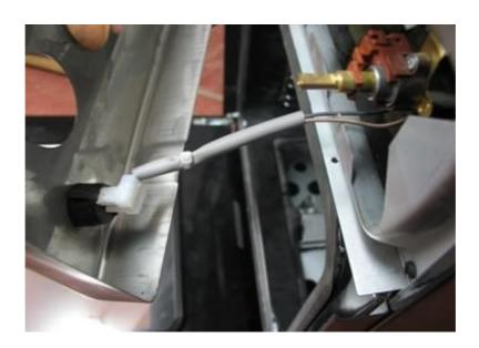
**2-**Remove the plastic contacts of wiring terminals ( with a nipper )
