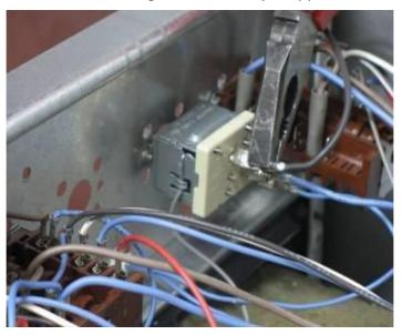
Unscrew the thermostat from the inner panel
