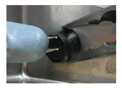
**4-**Insert a new button; set it appropriate into the hole.
