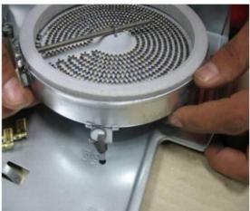
Put the heating element on a smooth surface, then take off the heating element assembly spring and bracket.
