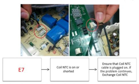
E7 error is showed when coil temperature could not be measured. Check the cable and plug in.
