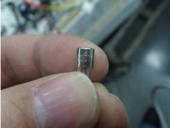
6 4-way valve"DHF-5 240V~ 6.5W TUV" is not same as the ones"DHF-5 230V 6.5W TUV" in CDF
