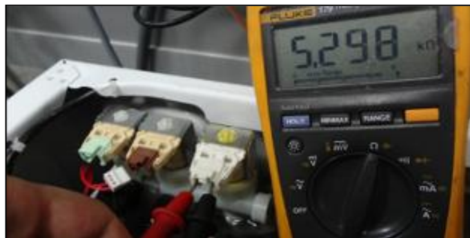
Dryer Valf Control
