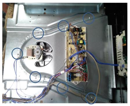
Detach the nut by turning counterclockwise
