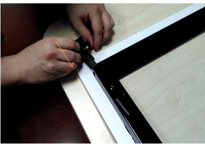
Disassemble removable inner glass spring as below,
