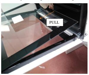
Unscrew as below to disassemble door profile.
