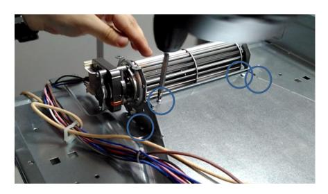
Pull the motor to below direction and remove
