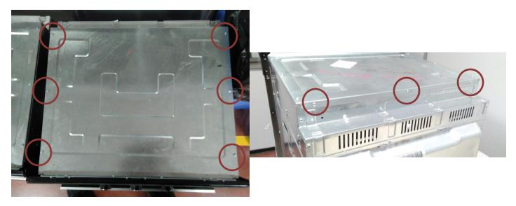
For disassembling raer panel, unscrew which are shown inside circles. Also, unscrew the screws right side of rear panel which is placed same locations
