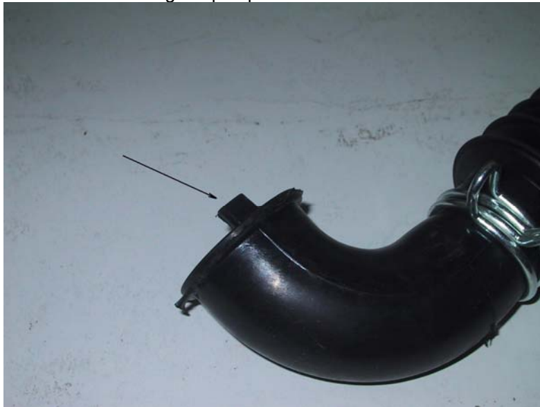
Photo of bellows showing the pump side
