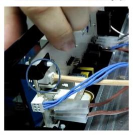
2. Remove PT1000 from Visio touch and unscrew the bulb from cavity as below.
