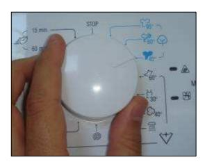
While pressing 1. function button, change position of the third to second, and release the 1. function button <u>immediately</u>.
