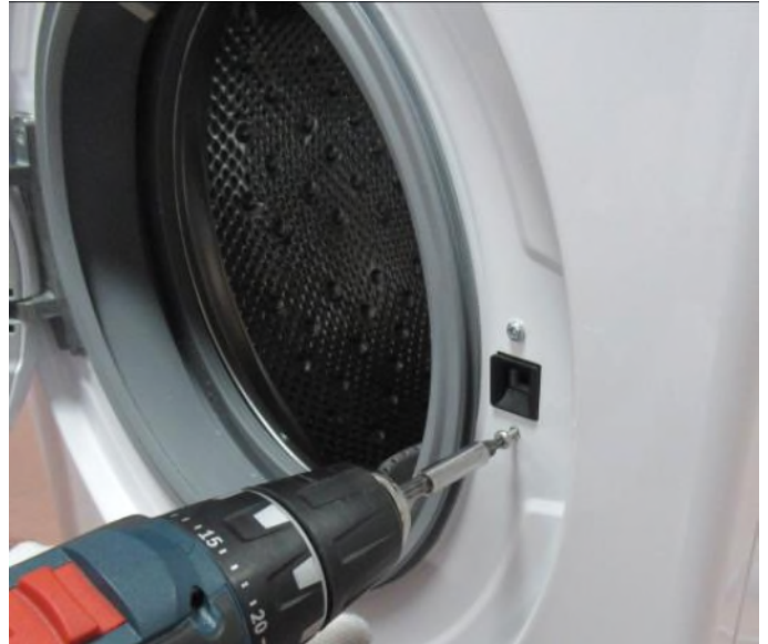
3.8 Remove the screws fixing the door lock.
