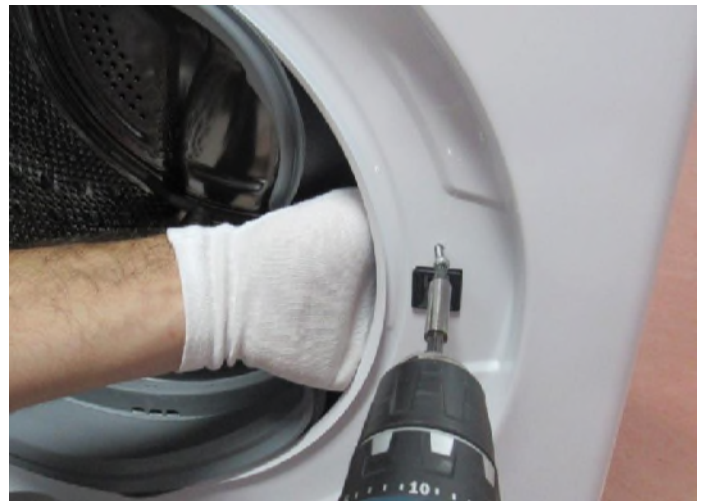
4.6 Tighten the door lock screw
