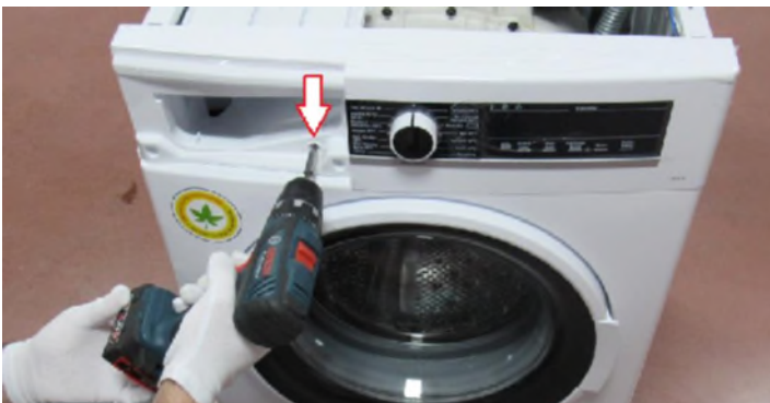
4.5 Tighten the screw which fixes the control panel to the front panel.
