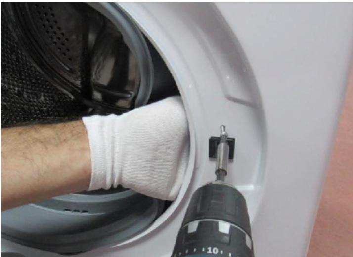
4.2 While supporting the door lock by hand, tighten the screws fixing the door lock.
