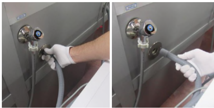
1.3 Disconnect the drain hose
