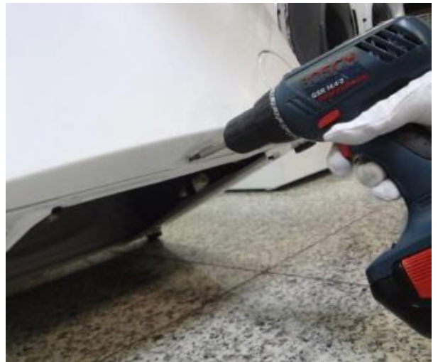
Tighten the screw fixing the front panel at the bottom
