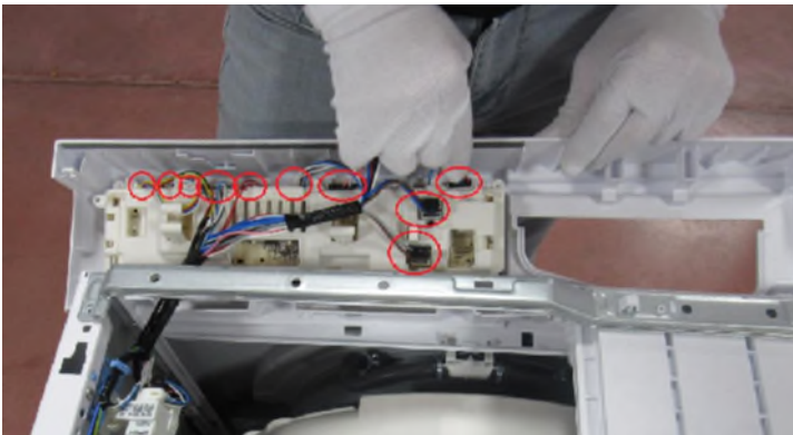
3.6 Remove the sockets on the card.
