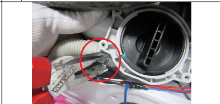
2.15. Remove clamp holding twinjet hose by using a plier.
