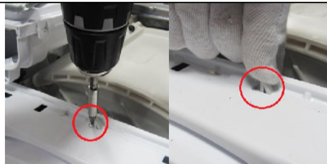
2.5. Remove the screw fixing twinjet elbow.
