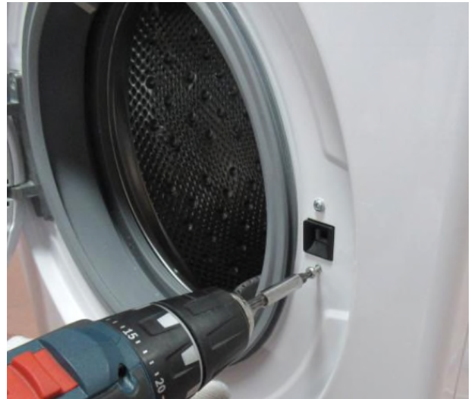
3.1 Remove the screws fixing the door lock.
