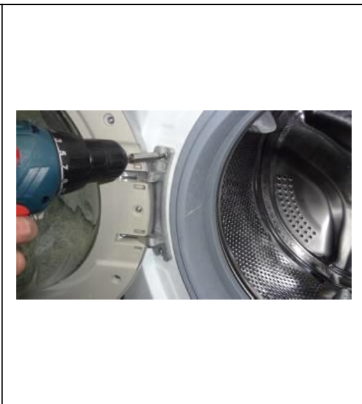
2.2. Remove the door hinge screws by using a Tx25 head screwdriver
