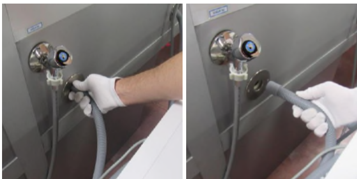
Disconnect the drain hose
