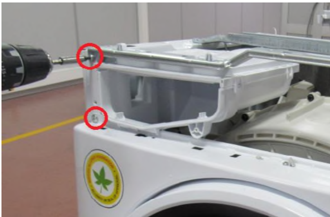
3.6 Remove the screw on support bracket and two screws fixing front panel to body
