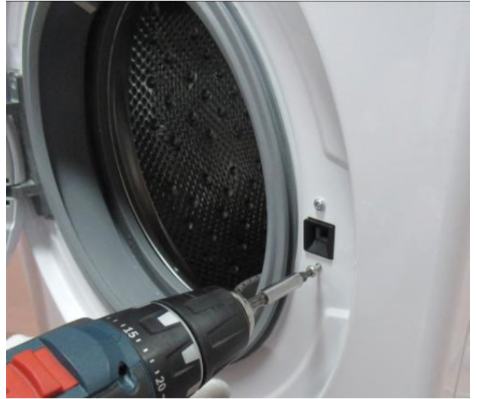
Remove the screws fixing the door lock.
