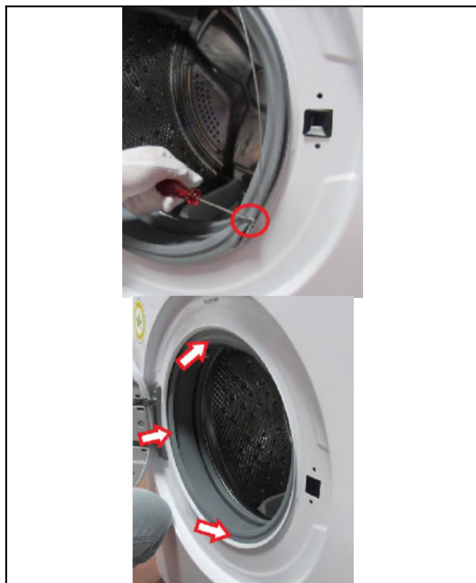
2.1. Remove the wire by using small screwdriver and push the seal to the inside
