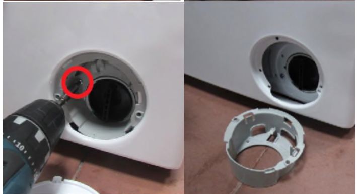
3.9 Remove the screw and plastic part located under the pump cover
