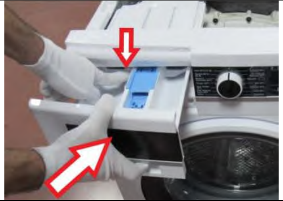
3.6. While pressing siphon cover keep pushing drawer to assemble it.
