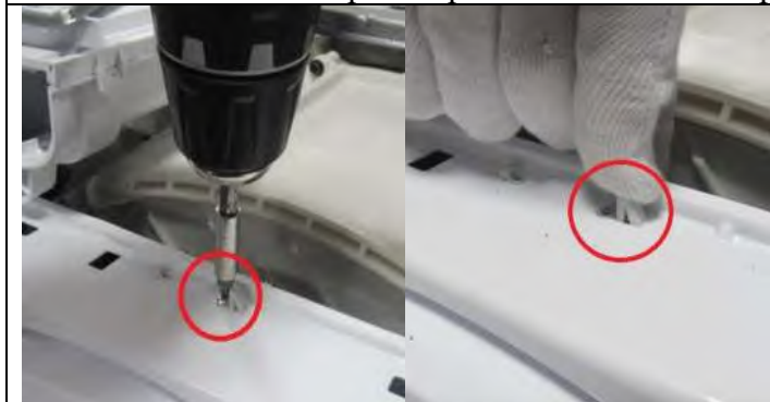
3.9.1. Assemble the twinjet elbow to the front panel
