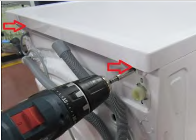
2.1.1 Remove two screws that fix the top-plate at the back.
