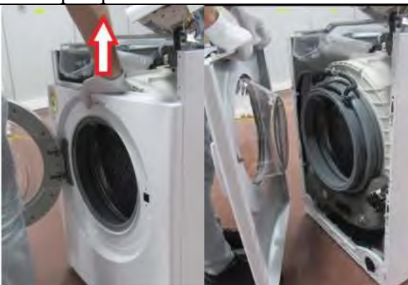
2.7.2 Pull up and remove the front panel.
