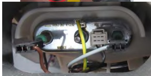
3.4. Connect the all sockets on the heater
