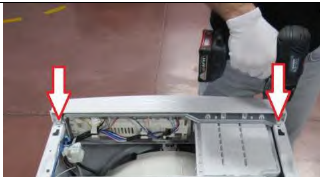
3.12 Tighten two screws fixing control panel.
