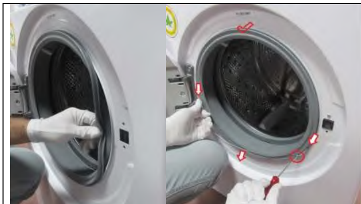
3.6.1. Pull the tub bellow seal to the outside and assemble the wire by using small screwdriver
