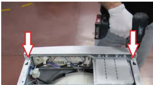
3.10. Tighten two screws fixing control panel.
