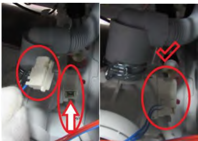
3.3. Connect the drain pump connector
