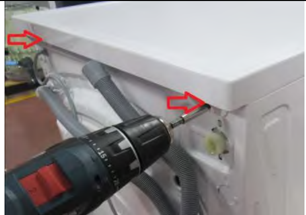
3.8 Tighten two screws that fix the top-plate at the back.
