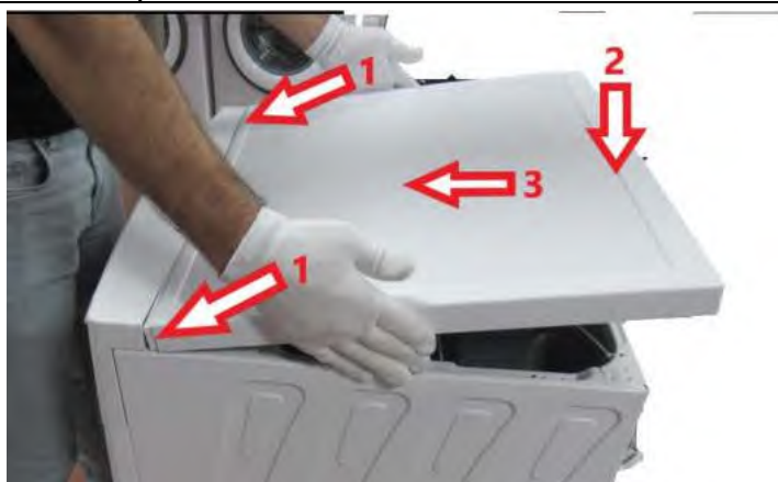
3.13. Fit the upper tray according to movement above
