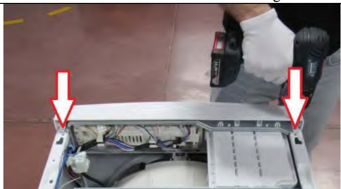
3.4 Tighten the two screws on control panel.
