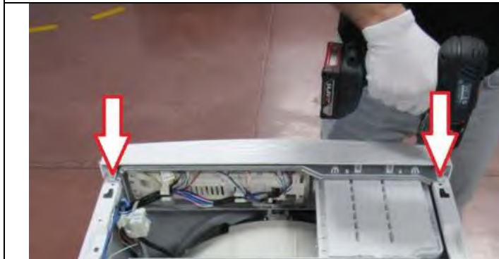
3.11.1 Tighten two screws fixing control panel.
