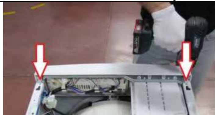
3.4 Tighten the two screws on control panel.
