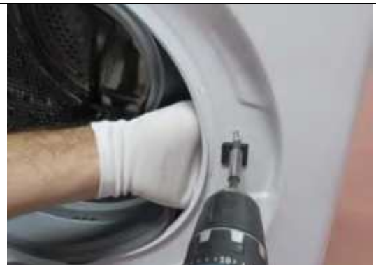
3.6. Tighten the door lock screw
