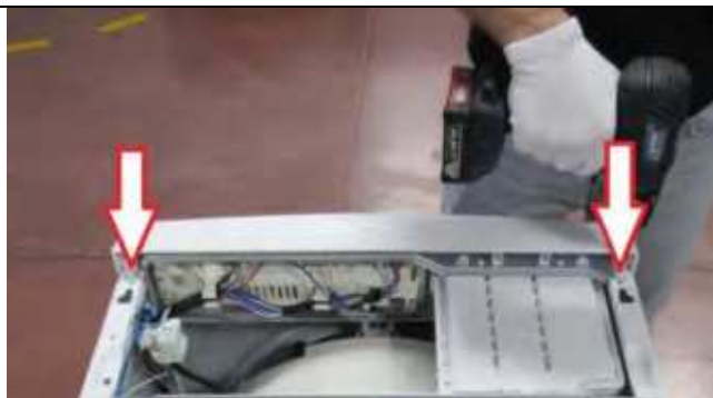
3.12 Tighten two screws fixing control panel.
