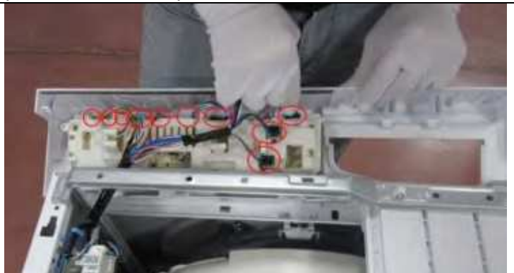
2.4.1 Remove the sockets on the card
