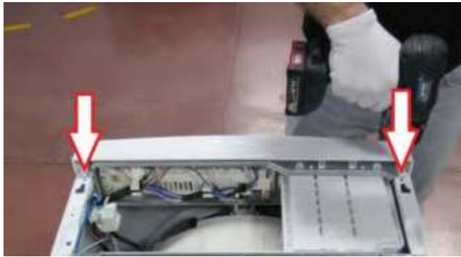
3.10. Tighten two screws fixing control panel.
