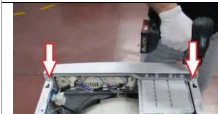
3.11.1 Tighten two screws fixing control panel.
