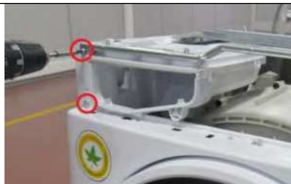
3.10.1 Tighten the screw on support bracket and two screws fixing front panel to body
