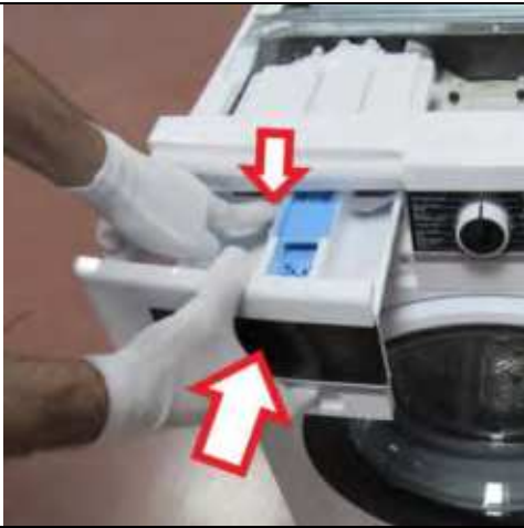
3.14 While pressing siphon cover keep pushing drawer to fit it
