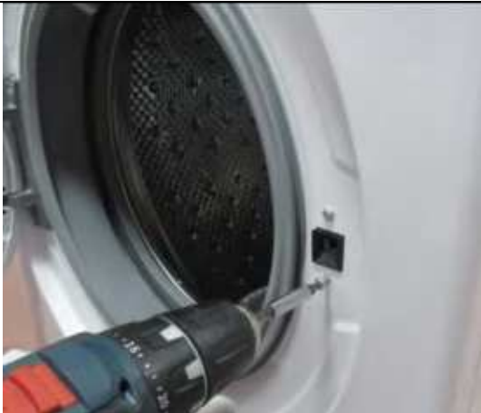
2.4.4 Remove the screws fixing the door lock.
