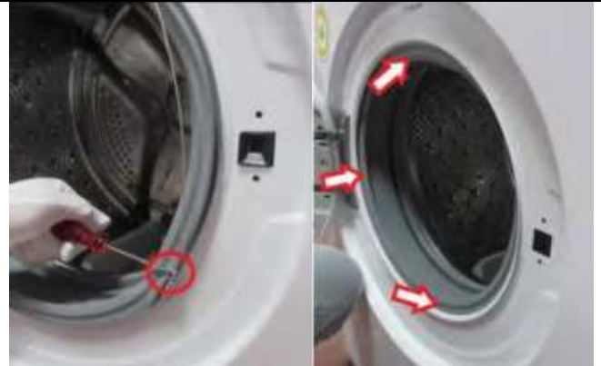
2.7.1 Remove the wire by using small screwdriver and push the seal to the inside
