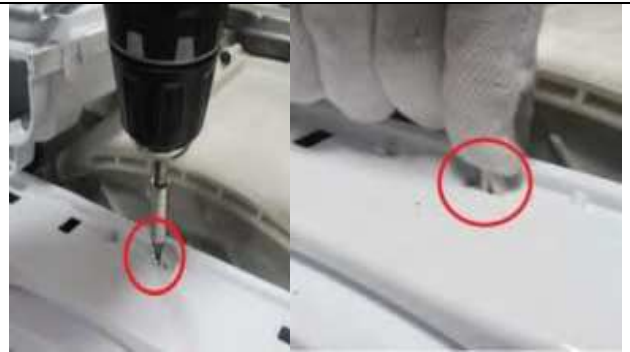
2.4.3 Remove the screw fixing twinjet elbow and the twinjet elbow later
