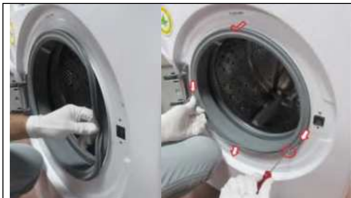
3.7 Pull the tub bellow seal to the outside and assemble the wire by using small screwdriver
