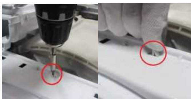
3.8. Assemble the twinjet elbow to the front panel
