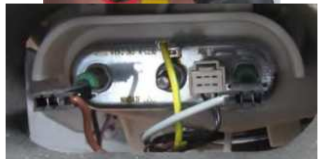
3.4. Connect the all sockets on the heater
