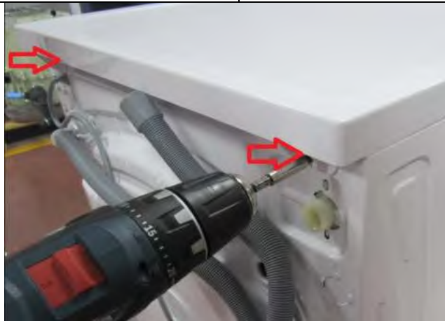
3.16 Tighten two screws that fix the top-plate at the back.
