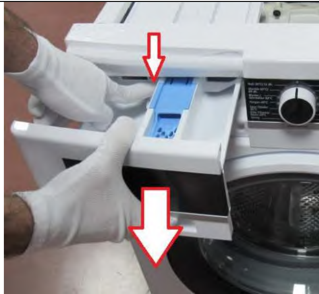
2.2.1 While pressing siphon cover keep pulling drawer to remove it.
