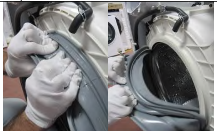
2.9.2 Hold the tub bellows seal and gasket-body fixing spring together, and pull them out.
