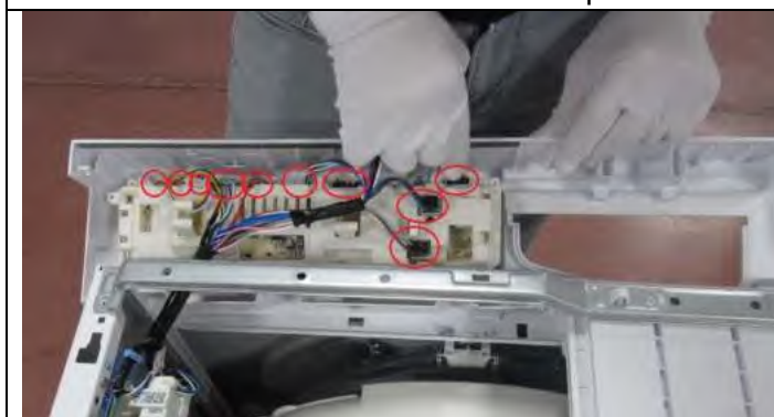
3.3. Connect the all sockets on the card according to the wiring diagram.
