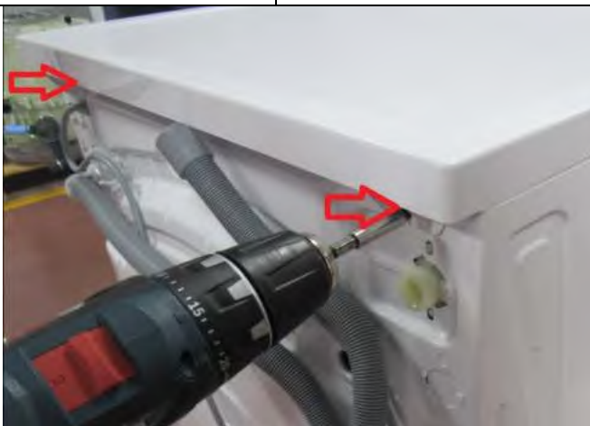
3.14. Tighten two screws that fix the top-plate at the back
