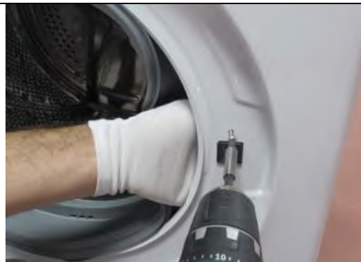
3.6. Tighten the door lock screw
