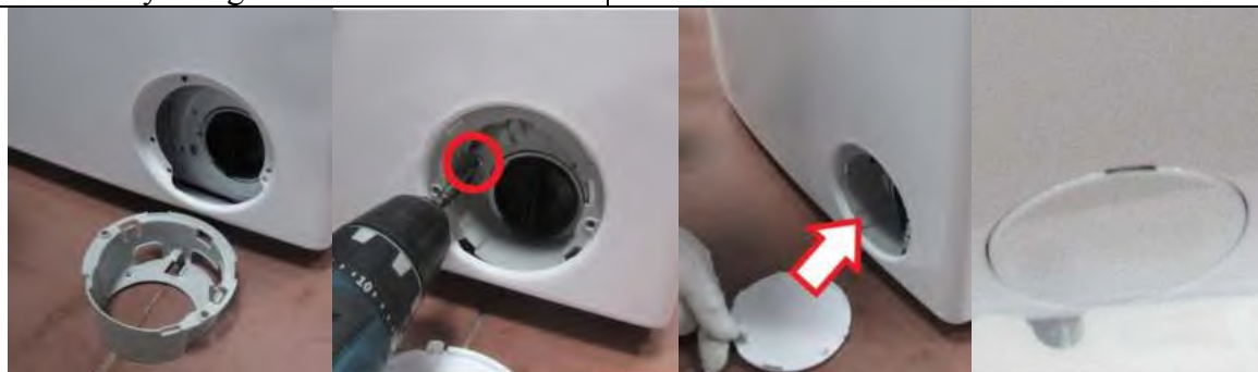
3.7. Tighten the screw and plastic part located under the pump cover
