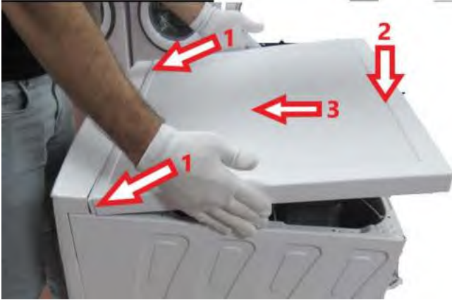
3.7. Fit the upper tray according to movement above
