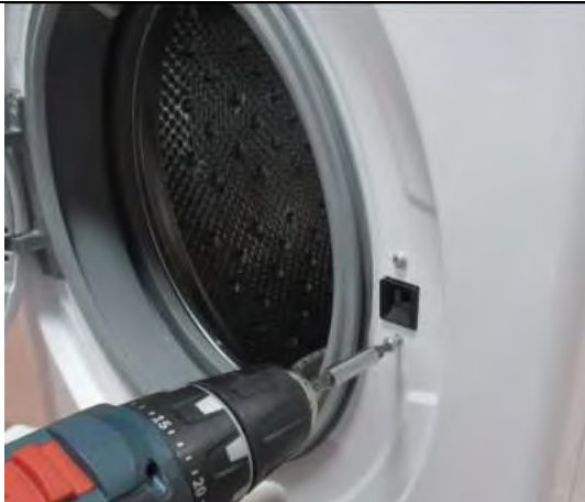
2.4.4 Remove the screws fixing the door lock.
