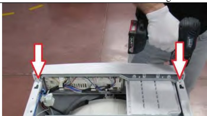
3.4 Tighten the two screws on control panel.
