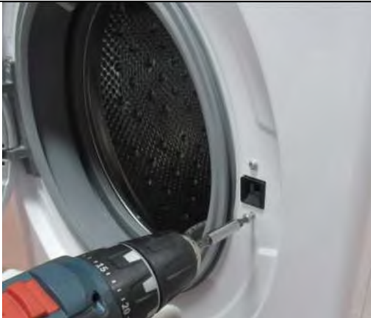
2.4.4 Remove the screws fixing the door lock.
