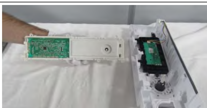
2.6.1 After releasing sockets, remove PCB box from its housing
