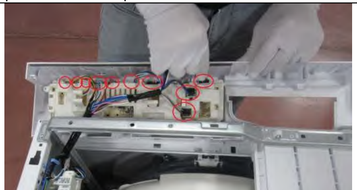
2.4.1 Remove the sockets on the card
