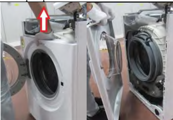
2.7.2 Pull up and remove the front panel.
