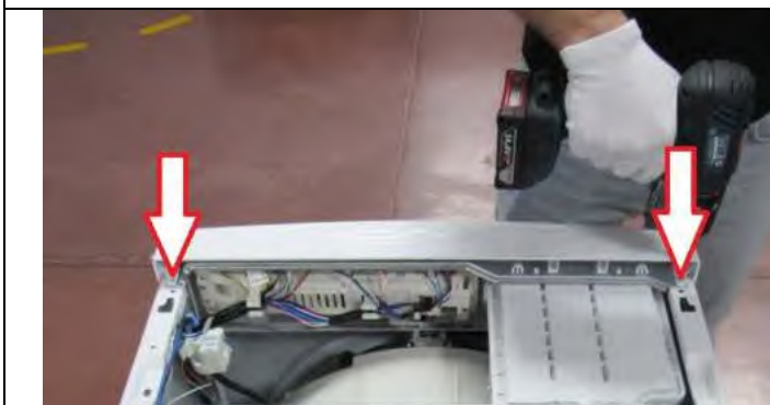
3.11.1 Tighten two screws fixing control panel.
