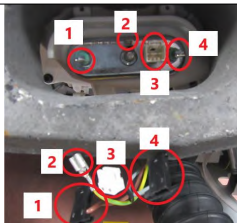
3.2. Fit the heater to the house well
