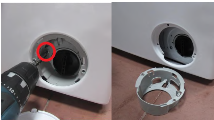
2.6.1 Remove the screw and plastic part located under the pump cover
