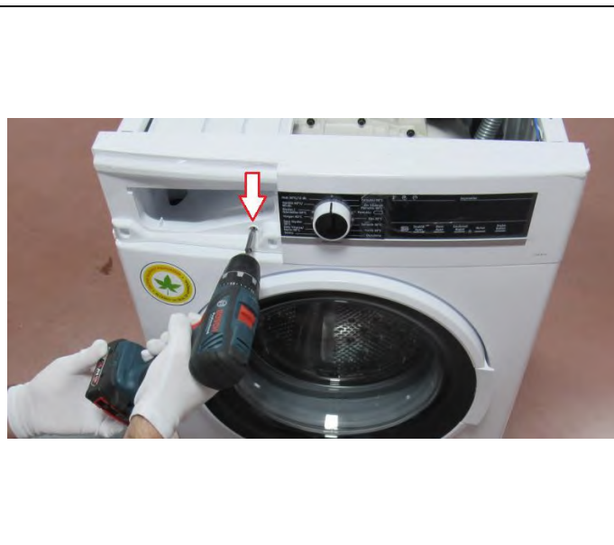
2.3.1 Remove the screw, which fixes the control panel to the front panel.
