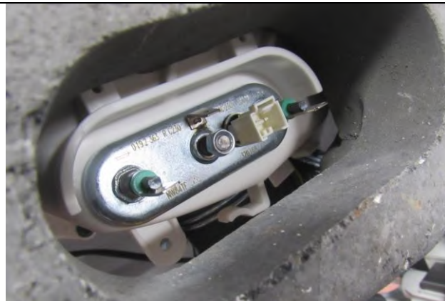
3.2. Fit the heater to the house well
