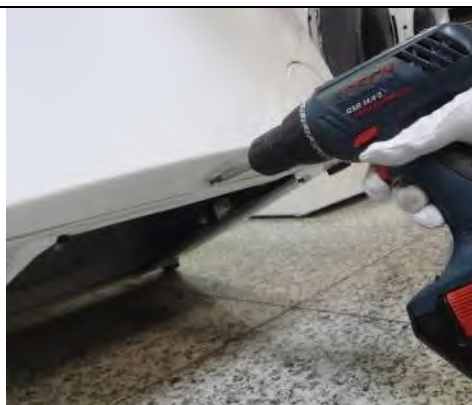
3.7.1 Tighten the screw fixing the front panel at the bottom
