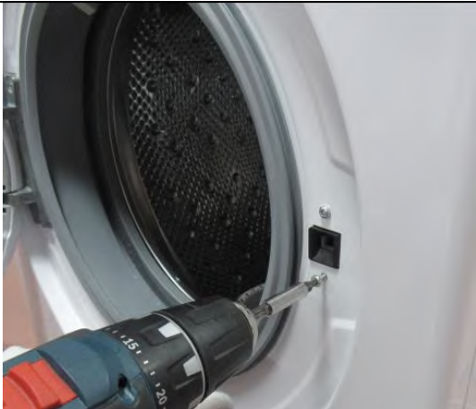
2.4.4 Remove the screws fixing the door lock.
