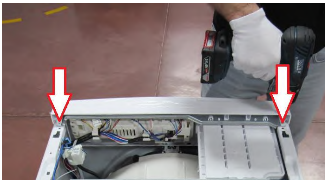
3.10. Tighten two screws fixing control panel.
