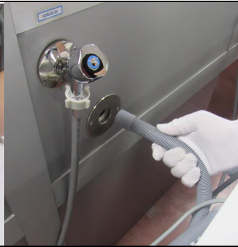
1.3. Disconnect the drain hose
