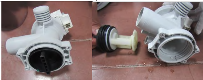
2.10.2 Remove the drain pump and change with the new one
