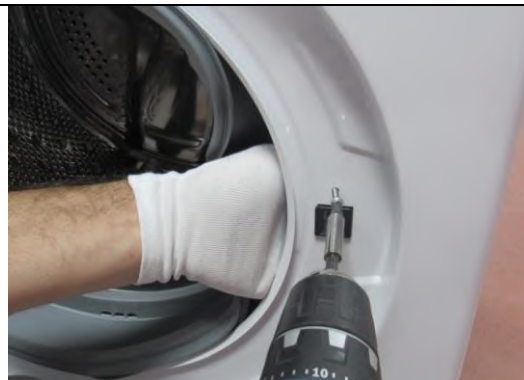
3.6. Tighten the door lock screw
