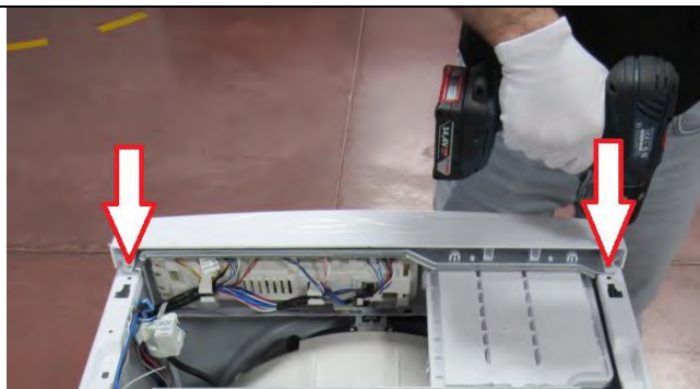
3.12 Tighten two screws fixing control panel.
