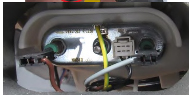
3.4. Connect the all sockets on the heater
