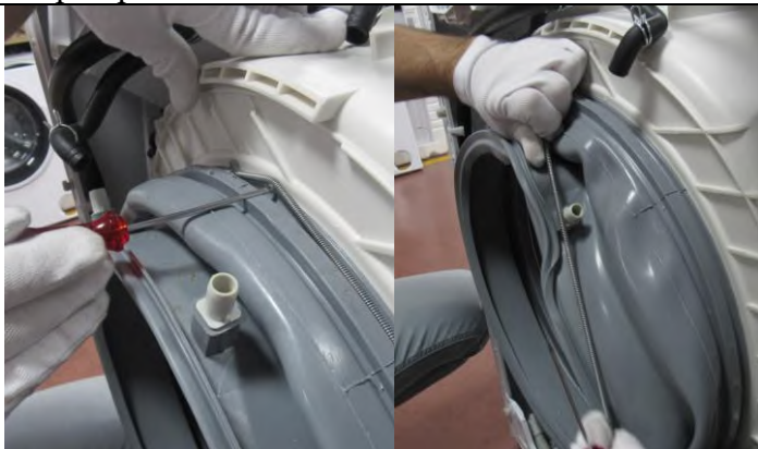
2.9.1 Remove the tub gasket clip by using small screwdriver.
