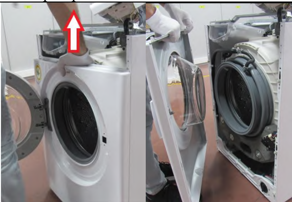
2.7.2 Pull up and remove the front panel.
