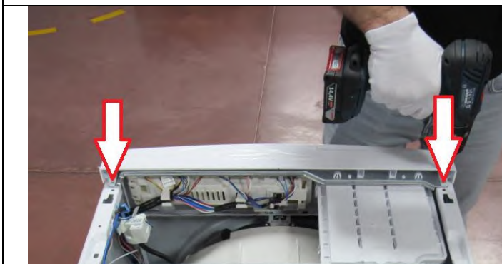
3.11.1 Tighten two screws fixing control panel.
