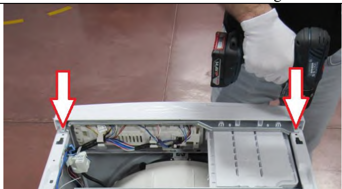
3.4 Tighten the two screws on control panel.
