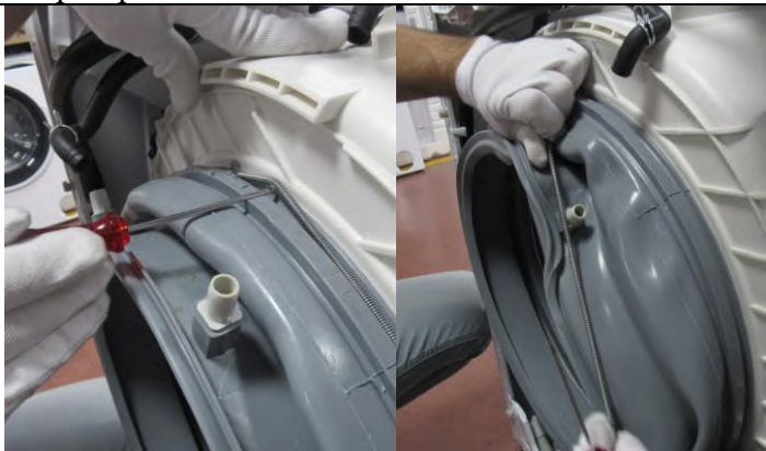
2.9.1 Remove the tub gasket clip by using small screwdriver.
