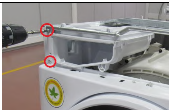
3.11. Tighten the screw on support bracket and two screws fixing front panel to body
