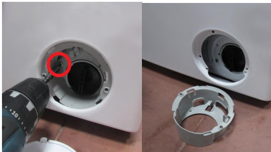
2.6.1 Remove the screw and plastic part located under the pump cover
