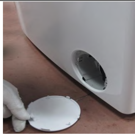
2.5.1 Remove the pump cover
