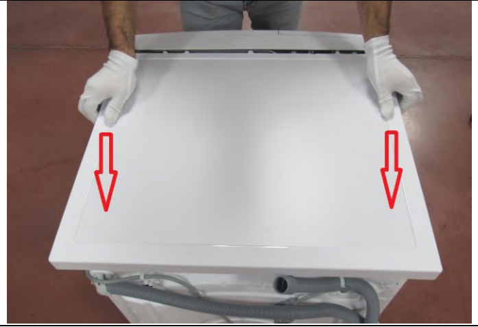
2.1.2 Push the top-plate back and pull it up.
