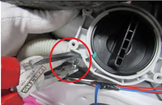
2.9.3 Remove clamp holding twinjet hose by using a plier.
