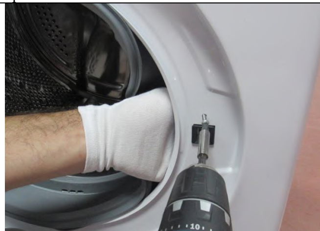
3.5.1 Tighten the door lock screw
