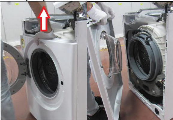
2.7.2 Pull up and remove the front panel.
