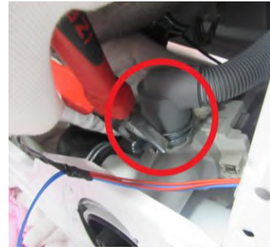
2.9.2 Remove clamp holding drain hose by using a plier.
