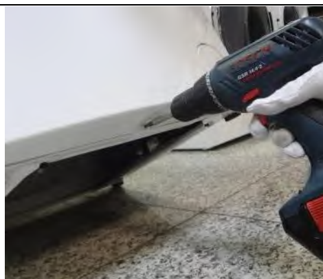
3.8. Tighten the screw fixing the front panel at the bottom
