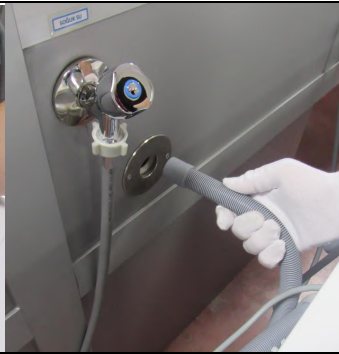
1.3. Disconnect the drain hose
