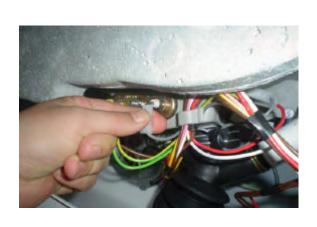
Remove one nut fixing the resistance.
