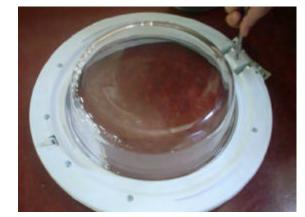
Remove the door inside plastic as it is showing the picture.
