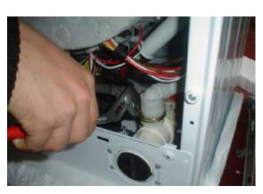
Remove pipe clip fixing the tub outlet hose.
