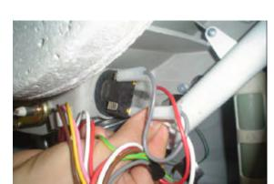
Remove the thermostat as it is showing the picture.
