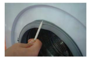
Remove the gasket-body fixing string.
