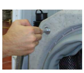
Hold the gasket and gasket-body fixing spring together, and pull them up.
