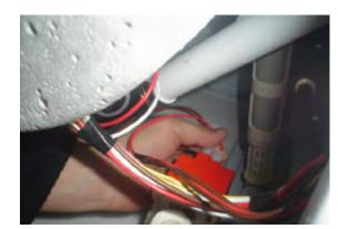
Remove four screws fixing the pump motor.
