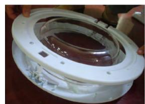
Remove the door hinge as it is showing the picture.
