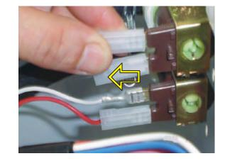
Remove the valve connection.
