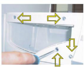
Remove two screws fixing the control panel.
