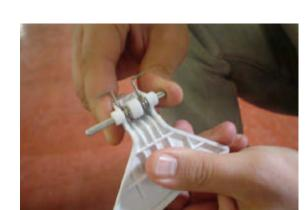
Remove the door handle spring as it is showing the picture.
