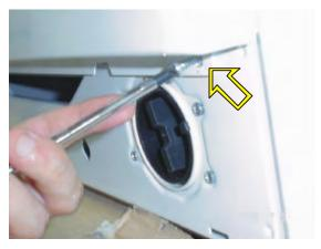
Remove two screws fixing the door lock.
