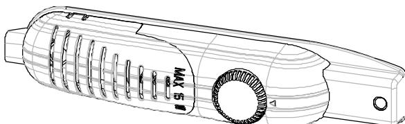
The fridge freezer thermostat automatically regulates the inside temperature of the compartments. By rotating the knob from position 1 to 5, colder temperatures can be obtained.
