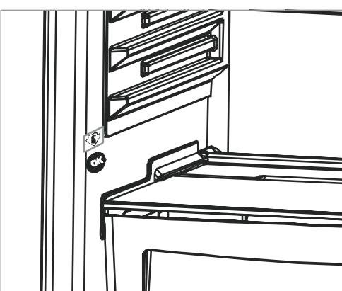
To be sure to have a low temperature in this area, make sure the shelf is located at the level of this symbol, as shown in the illustration.
