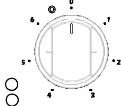
Dual and oval heaters have two heating zones. To activate the outer zone of a dual/oval heater, turn the knob to
