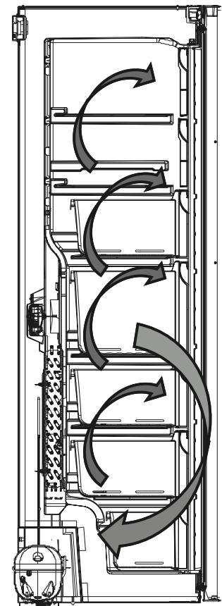
The situation is completely different in no-frost freezers. Dry and cold air is blown into the freezer compartment homogeneously and evenly from several points via a blower fan. Cold air dispersed homogeneously and evenly between the shelves cools all of your food equally and uniformly, thus preventing humidity and freezing.
