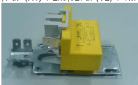
Condensateur Anti-parasite 0,1 \mu\text{F} (X1) + 2 \times 0,027\mu\text{F} (Y2) + 1\text{M} \Omega
