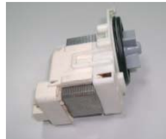
Pompe de vidange 30W – 17-21L/sec – 143ohm \pm 7\% - Protection thermique 120C°
