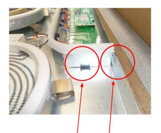
ENSURE THAT THE PCB PROTECTION SHIELD IS FITTED INFRONT OF THE SIDE LUGS AND INTO THE BASE TRAY SLOTS AS SHOWN TO PREVENT THE SHIELD FROM BEING PUSHED ONTO THE PCB.
