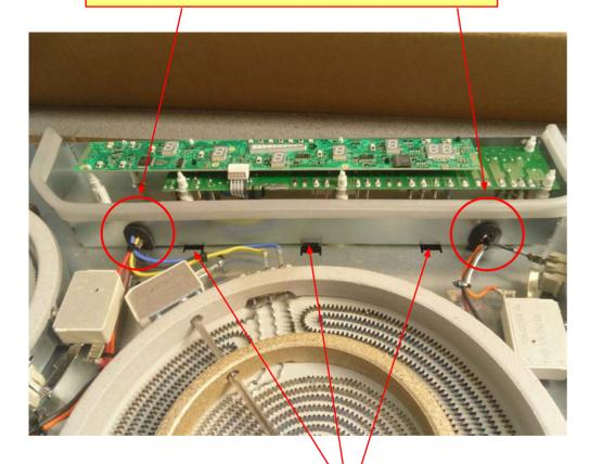
ENSURE THAT THE PCB PROTECTION SHIELD IS FITTED INFRONT OF THE TWO OUTSIDE LUGS AND BEHIND THE CENTRE LUG AS SHOWN ABOVE.
